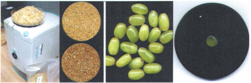
Figure 2.5. As the sample gets larger and more non-uniform, the approach is to average out the variation in single measurement or as a group.
