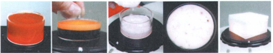
Figure 2.3. With translucent samples, it is necessary to control the thickness of the sample to make it effectively opaque for color measurement.
