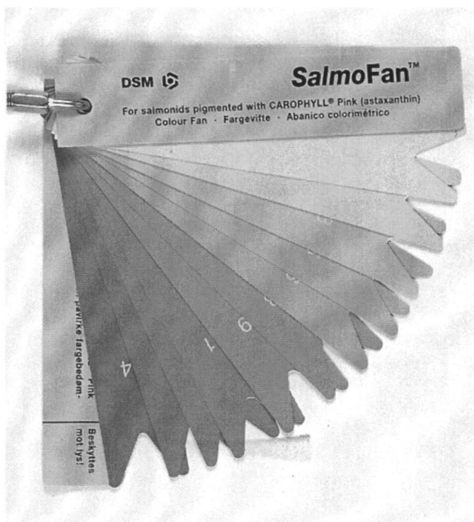
Figure 2. SalmoFan ™ used for evaluating color of salmon world wide. (See page 16 of color inserts.)
