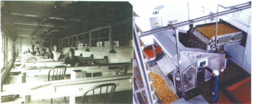
Figure 5.8. Hand and Automated Color Sorting
